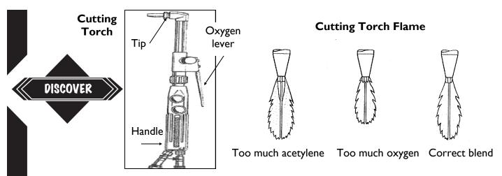
The flow pressures that we set on the oxygen and acetylene regulators will have to be changed when using the cutting attachment. For general cutting operations, a common pressure of 3-5 p.s.i. acetylene and 25 - 35 p.s.i. oxygen will work. If the cutting tip is clean and working properly, this will allow you to cut regular steel up to 3/8 inch (10mm) thick. If the material is thicker, you may need to increase the oxygen pressure or tip size.
