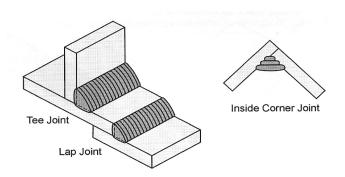
**Fillet** - The fillet weld is generally a layer of weld to fill in corners created in joints. The weld looks like a triangular shape. It is most commonly used on lap, tee and corner joints.
